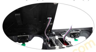
The back of the module is fixed magnetically close to the cabinet;
