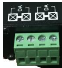
DALI signal line interface, the left two ports are one signal, the right two ports are another signal
