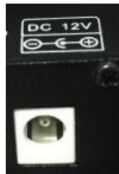
Power interface, can input DC12 to 48V;
