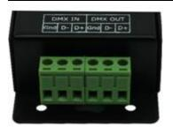
**DMX IN**: input interface of DMX signal, D+ should be connected with positive of signal, D- connected with negative of signal, Gnd connected with ground.
