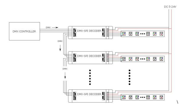
**Double power connect single signal line strip condition:** if the V+ voltage light signal is single, you need to connect another power supply.
