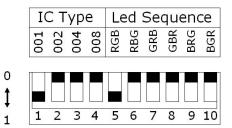
IC type: selection of light type. The accumulation of first four DIP is 1\*1+2\*0+4\*0+8\*0=1, lookup the table, you can find it is LPD6803.
