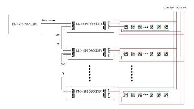
**Double power connect double signal line strip condition:** if the V+ voltage of strip is not the same with controller input voltage and light signal is double, you need to connect another power supply.
